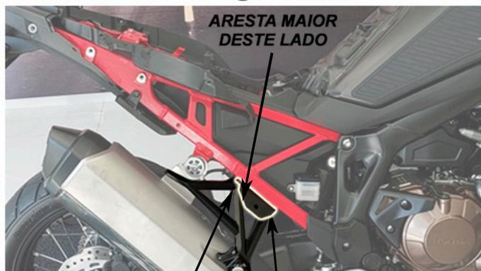
REMOVER O SUPORTE DA PEDALEIRA E PRENDER O FIXADOR FRONTAL (D) ENTRE ELE E O CHASSI USANDO OS PARAFUSOS ORIGINAIS (VISTA LD)
